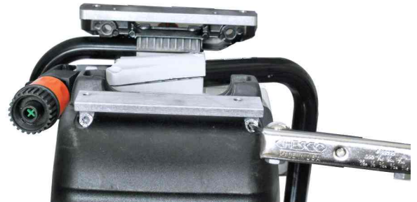
Fig. 2 — Remove filter cover screws (2), install rear mounting bracket, reinstall the cover screws and tighten securely.
