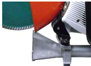
Fig. 5 — Adjust the saw's blade guard to the top of the Dust Director.
