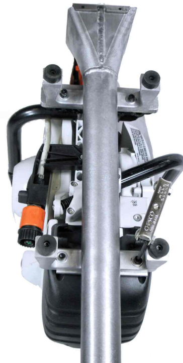
Fig. 4 — Installation of Dust Director onto Mounting Brackets
