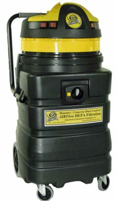
**Airtight Sealed Collection Tanks** - Dust Director® Vacuums ensure you against Dust Exhaust or Leakage. By preventing even the slightest loss or escape of dust, suction power also increases. Each Dust Director® Vacuum has a poured in-place urethane gasket beneath its motor head to create a positive airtight seal between the motor head and its collection tank (picture, left).
