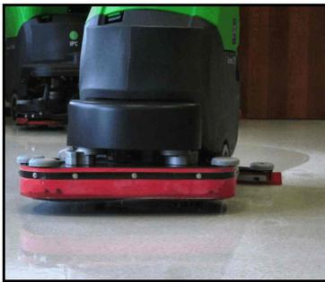
**Diamapad System - Concrete Grinding, Polishing, Coatings Removal, Maintenance.** For the DIY and Floor Professionals - Completely transform a worn, damaged, rough finish or mastic covered concrete floor using a standard low-speed rotary swing machine or an automatic floor scrubber. No special pads, holders or drivers are use - simply press a Diamapad onto the machine's own velcro pad driver.
