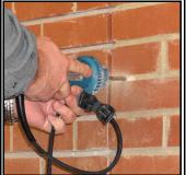
Finishes the cut where a diamond blade can't: - Inside wall corners, both horizontal & vertical
