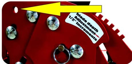
Pull Lift Arm back and install the locking pin in the above position when the saw is in operation.
