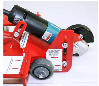
**Fig. 7** Grinder attachment bolts are also use for blade depth-of-cut. Rear eye-bolt with cable tie helps to secure the barrel of the angle grinder.
