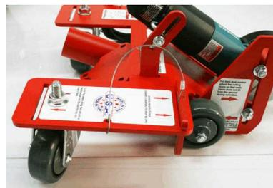
**Fig. 9** Insert the U-Shape Wheel Locks in the slots provided behind from the wheels to allow the casters to swivel freely while following cracks. Front wheels are adjustable by loosening the nuts - Maintain 1/4" clearance between the floor and the saw's frame.
