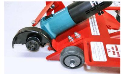
**Fig. 6** Attachment of Angle Grinder & Brackets to Saw.
