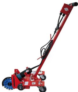
6" Dustless Crack Chasing Saw Cutting (not dustless)
