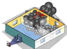
**Positive Pressure Ventilation (PPV)** - In a typical PPV application, the fan is placed about four to ten feet from the doorway of the structure and is positioned so that the cone of air produced by the fan completely seals the opening.
