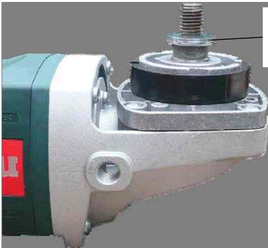
Adjust the height of the diamond cup wheel with the spacers (included with a Surface Dust Guard) or the inner blade clamps (included with the angle grinder.)
