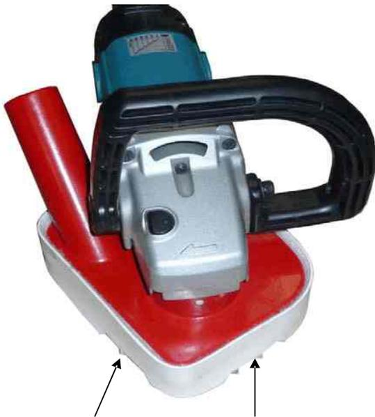
The diamond cup grinding wheel will extend past BOTH edging flats on the Surface Dust Guard
