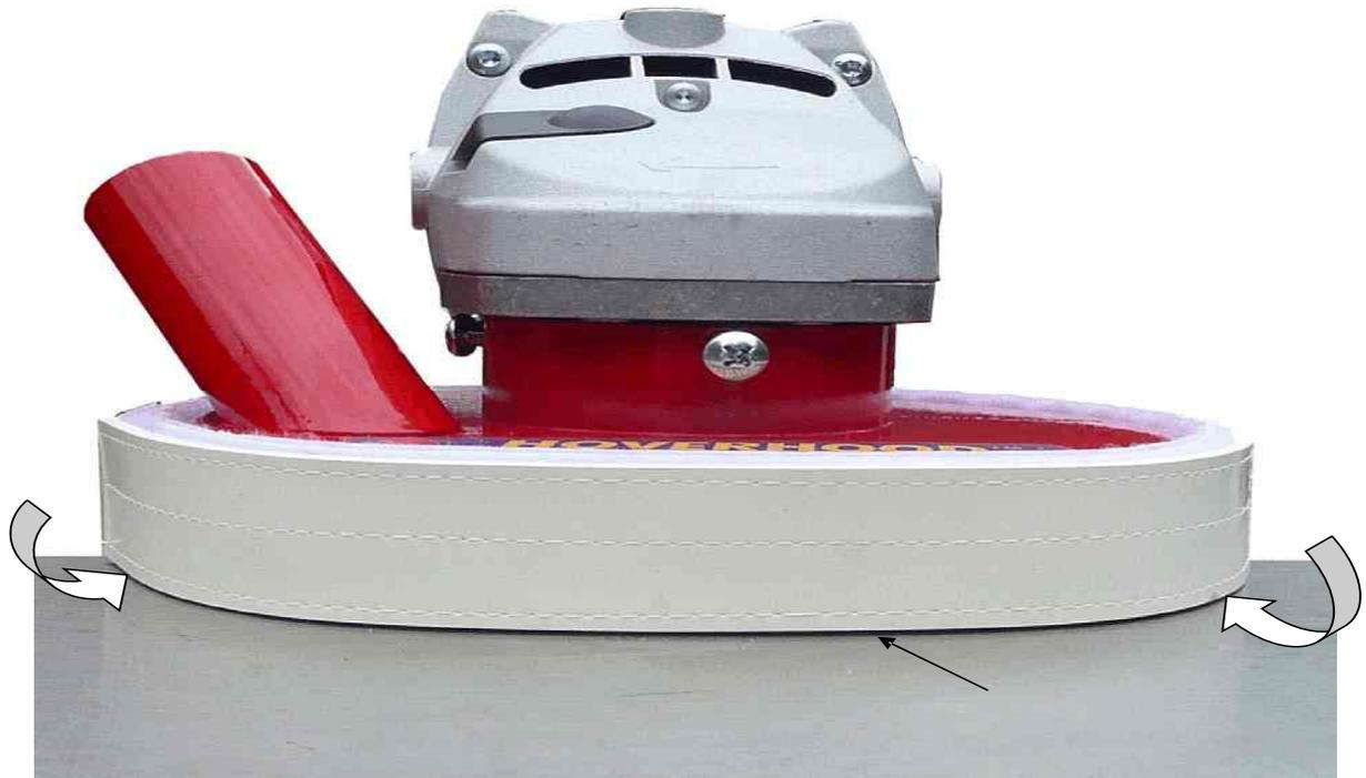
The strong airflow underneath the seal is what picks up dust on the floor as the Surface Dust Guard passes over, leaving the floor clean. Be sure to leave a small gap between the seal and the floor.
